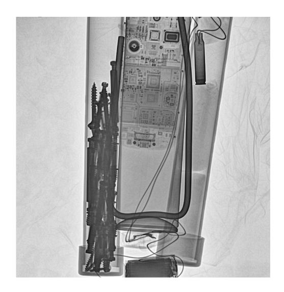
Sample image taken with XR150 20V (15 pulses) on SOSTÓS panel from 1 meter.
