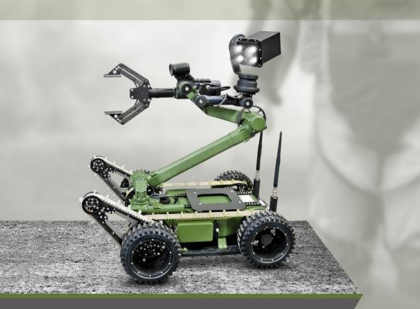
PIAP FENIX® robot is easy to transport – owing to its small size and low weight it can be carried in a backpack.
